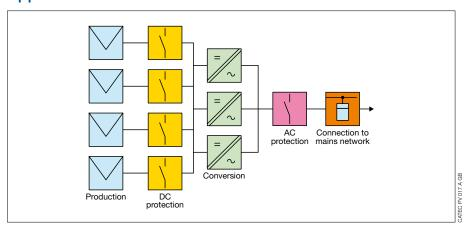
SIRCO AC load break switches are both reliable and flexible - with all the necessary credentials to perform in the most challenging operating conditions, such as solar systems equipped with strings inverters.
